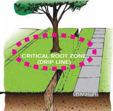
FENCE PROTECTION AROUND CRITICAL ROOT ZONE (DRIP LINE)
