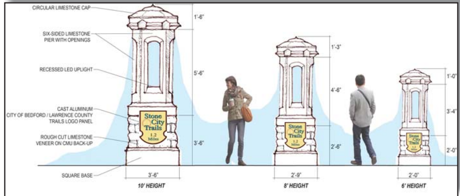
Branding: Stone City Lanterns - Trailside Markers
